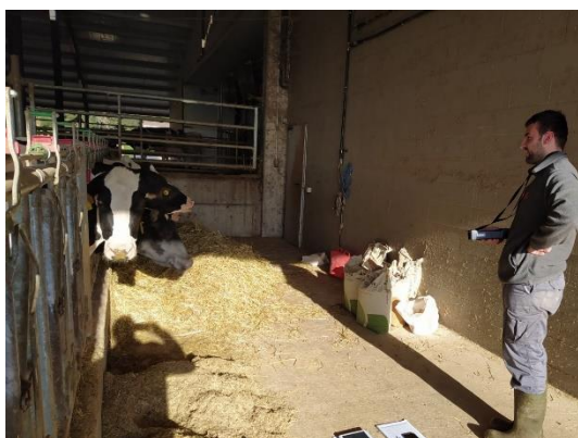
Methane measurements with the portable laser device - © Marta Terre
